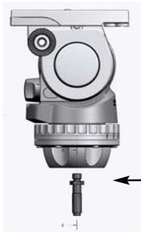
If you want to fit the FSB 8 onto a flat base, remove the threaded pin.
